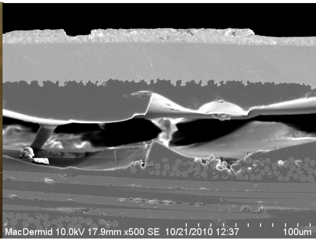
Fig. 6 – Delamination After Reflow
