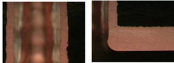
Figure 7. Cross Section of 0.25 mm Through Hole in 1.6 mm Panel Plated at 15 ASF
