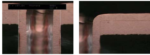
Figure 5. Cross Section of 0.20 mm Through Hole in 1.6 mm Panel Plated at 10 ASF, AR = 8
