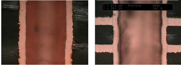
Figure 9. Cross sections of 0.20 mm Through Hole in 3.5 mm Panel Plated at 5 ASF
