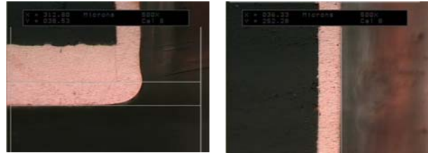
Figure 6. Cross Section of 0.50 mm Through Hole in 1.6 mm Panel Plated at 10 ASF
