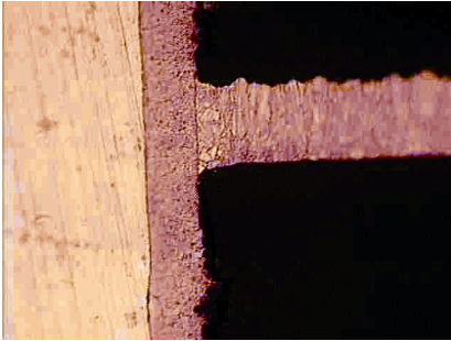
Figure 1 Direct metallization means copper plating directly to innerlayers
