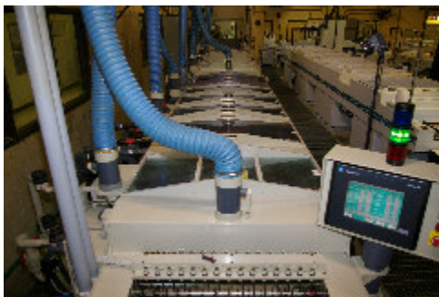
Figure 6 Enclosed conveyorized process line
