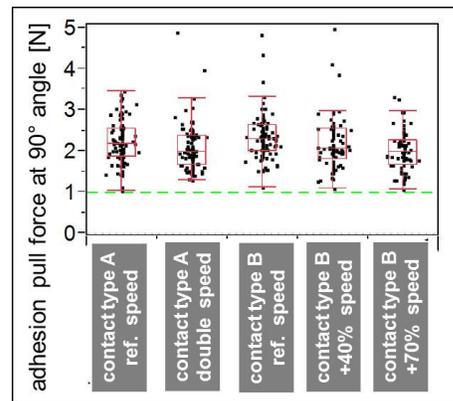
**Figure 2:** Comparative study of equipment and process modifications with respect to contacting the solar cell and passing a higher plating current through the solar cells while increasing in parallel the plating speed. No significant influence on the studied adhesion of interconnection ribbons soldered to the busbar regions has been observed.
