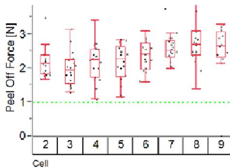
**Figure 4:** Pull test (90° pull angle) results after soldering interconnection ribbons to the busbars of mc-Si solar cells.
