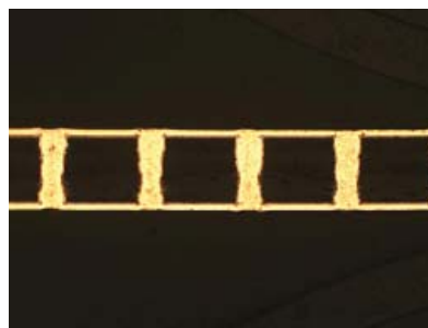
Figure 13 - 60 µm diameter filled up through vias in 200 mm thick substrate, DC plating
