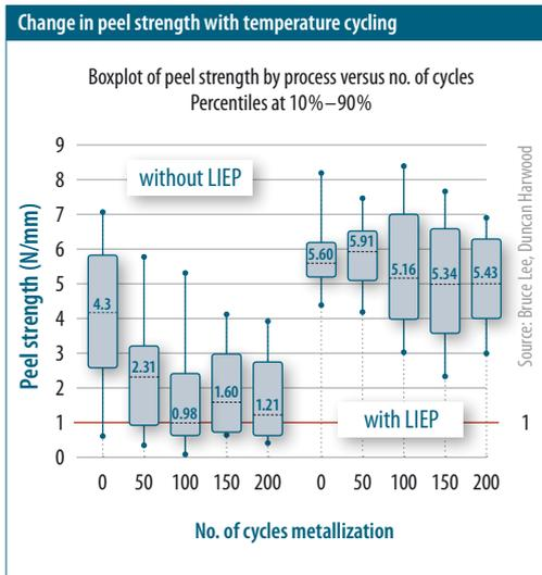
Figure 6: Measurement of peel strength as a function of temperature cycling shows a significant difference between cells manufactured with and without LIEP.
