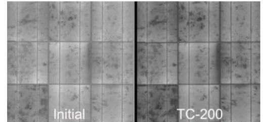
Figure 5: Module electroluminescence image with LIEP.
