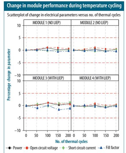
Figure 8: After 200 temperature cycles from -40°C to 85°C both groups of modules were comfortably within the IEC-61215 degradation limit of -5 percent.
