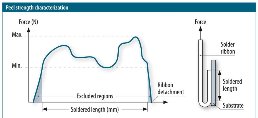
Figure 9: Measuring solder peel strength in a 180 degree configuration.
