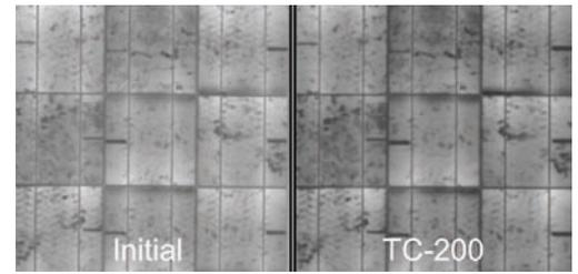
Figure 4: Module electroluminescence image without LIEP.
