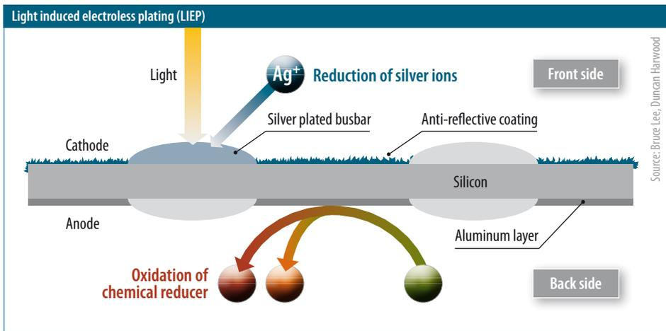
Schematic of the plating deposition reaction.
