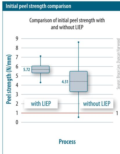
Figure 7: Comparison of the initial peel strength showed that the LIEP process not only produced higher median peel strength values but with less variation.
